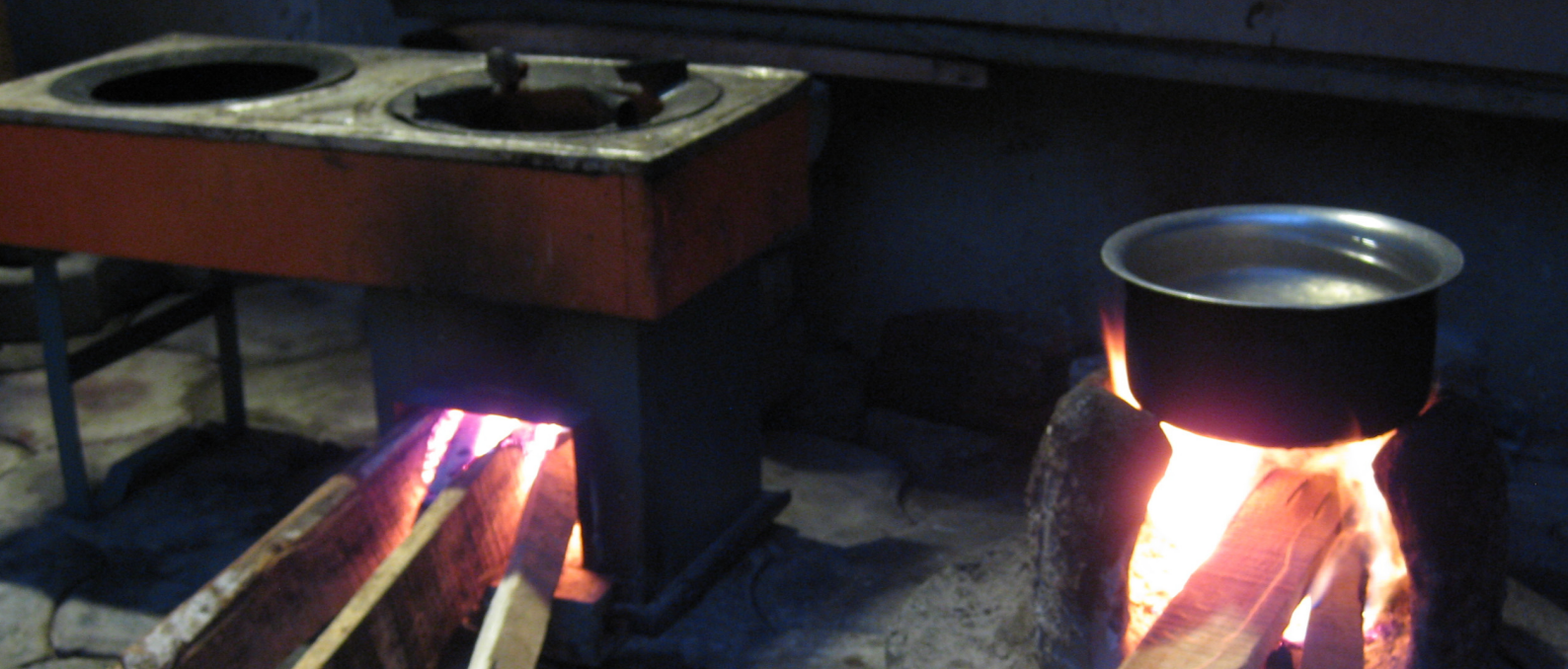
6: BoP tester's perceptions: The improved cookstove produced steady heat and was easier to ignite, but needed more fuel than her old chulha
