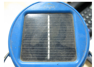
9: Without specific cleaning instructions, the users were unaware of how dust accumulation affected product performance
